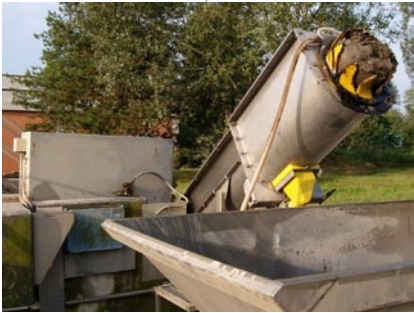
CPS Screw Compactor outlet plug
