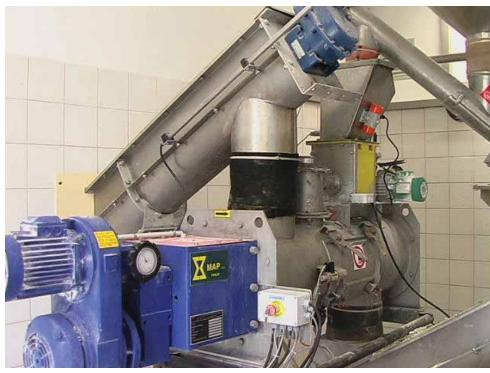
Shaftless Screw Conveyor and Micro-Batch Feeder feeding into Continuous Ploughshare Mixer
