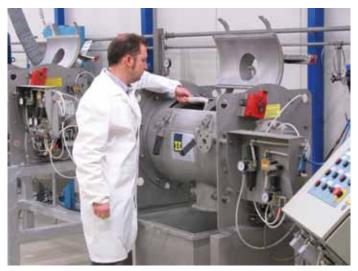
Mixing test on batch-type WBN Ribbon Blender
