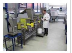
Accuracy test on MBF Micro-Batch Feeder
