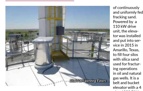
This heavy-duty mild steel centrifugal discharge Bucket Elevator made by WAM Texas with a 30 by 64-inch casing size has a nominal discharge height of 168 feet (51 metres). It elevates 472 tons per hour ply - 1000 PIW rubber belt and maxi-lift nylon elevator buckets. Along with the bucket elevator, WAM Texas also supplied VG 600 Slide Gates and SILOTOP® Venting Filters.
