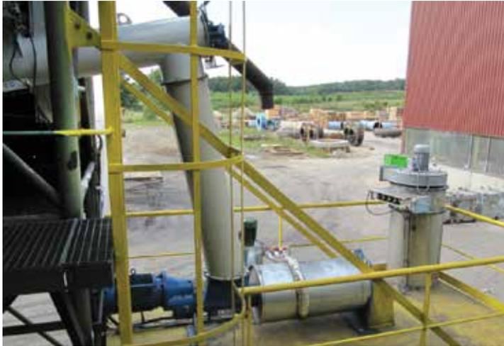
Installation with TP Screw Feeder, DUSTFIX® and WAMFLO® Dust Collector
