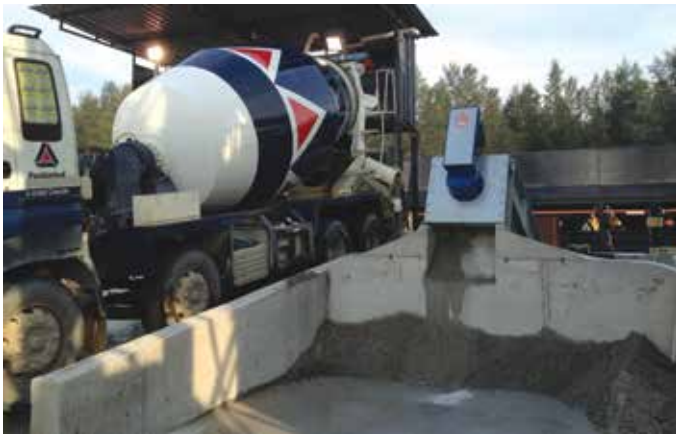
CONSEP® 5000 Concrete Reclaimer in operation in Singapore
