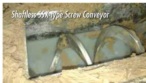
Shaftless SSX-type Screw Conveyor
