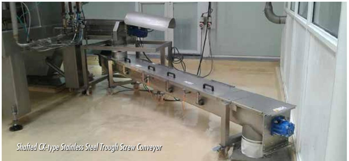
Shafted CX-type Stainless Steel Trough Screw Conveyor
