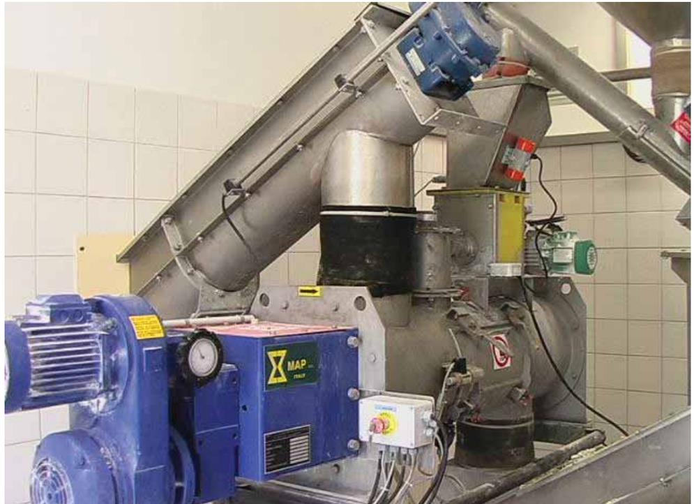
Shaftless Screw Conveyor and Micro-Batch Feeder feeding into Continuous Ploughshare Mixer
