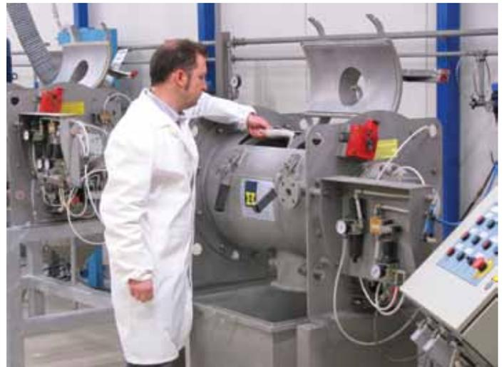
Mixing test on batch-type WBN Ribbon Blender
