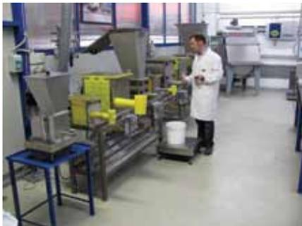
Accuracy test on MBF Micro-Batch Feeder
