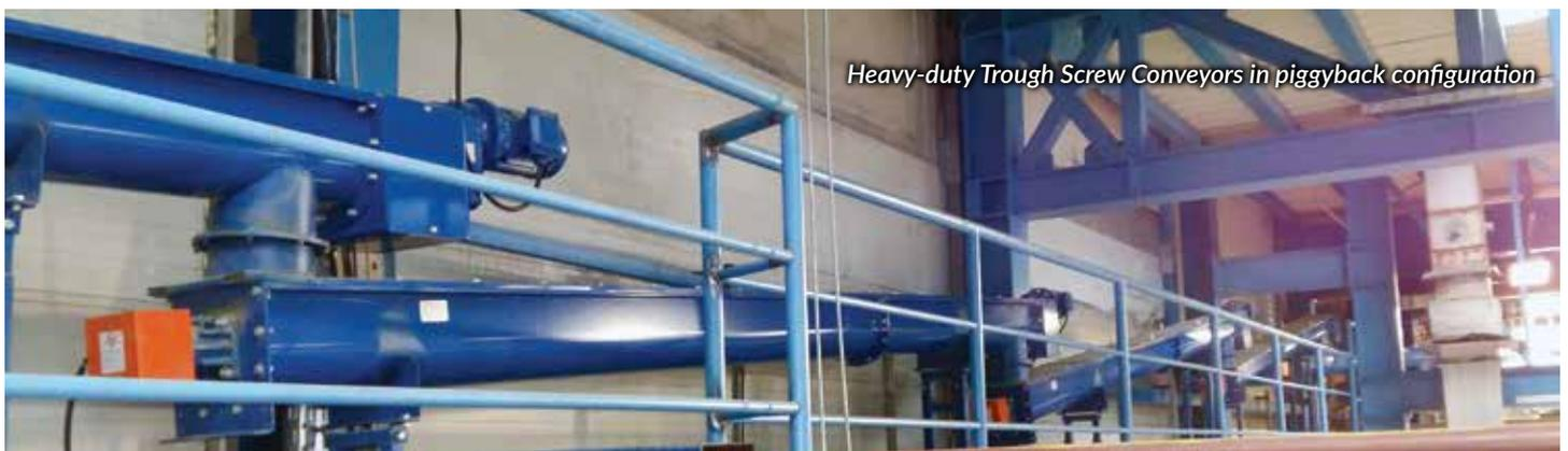
*Heavy-duty Trough Screw Conveyors in piggyback configuration*
