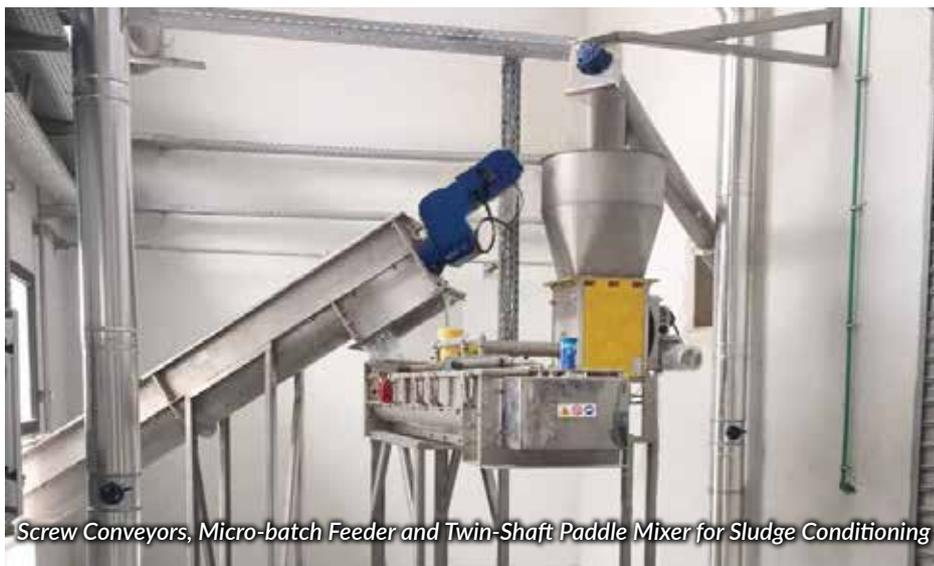
*Screw Conveyors, Micro-batch Feeder and Twin-Shaft Paddle Mixer for Sludge Conditioning*
