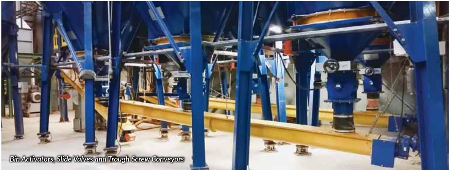
*Bin Activators, Slide Valves and Trough Screw Conveyors*
