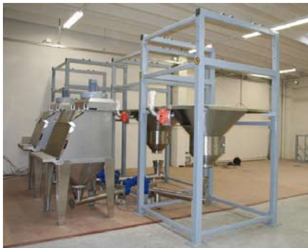
Powder Feeding Station for ADDCOMP
