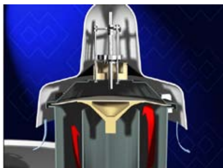
VHS in Excess Pressure Condition
