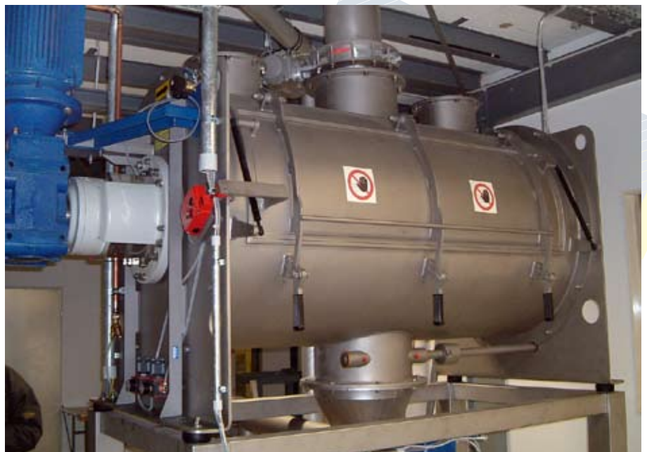
MAP® Batch-Type Ploughshare Mixer in DAIMLER foundry in Mettingen, Germany
