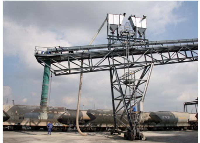
Air-slide De-dusting by WAMAIR® Dust Collectors
